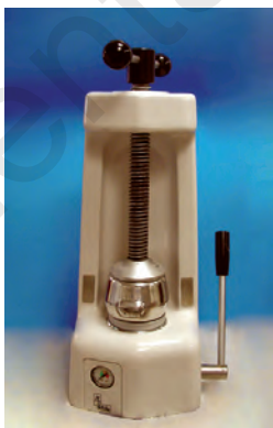
Figure 25.15: A hydraulic press (Kavo) is useful for trial and final closure of the flask. The pressure indicator dial indicates the pressure that is applied.
