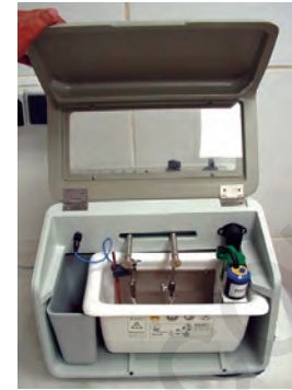
Figure 20.6: Electrolytic polishing unit.
