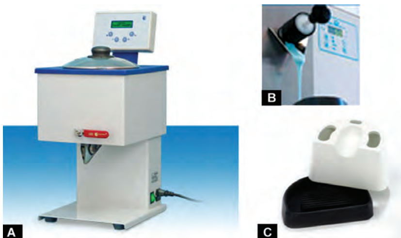
Figures 12.6 A to C: (A) The agar hydrocolloid duplicating machine liquefies the agar using heat. Rotating blades in the machine further break up the agar, (B) Liquefied agar is poured into a duplicating flask, (C) which holds the cast.
