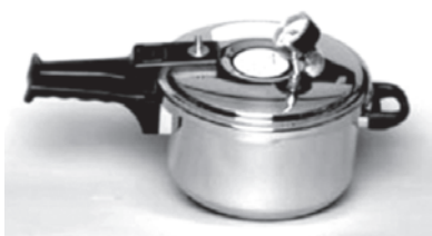
Figure 25.22: A pressure pot for further curing of chemically activated resins. It has a pressure dial (some models have a temperature indicator). Pressure is increased in the chamber using compressed air.
