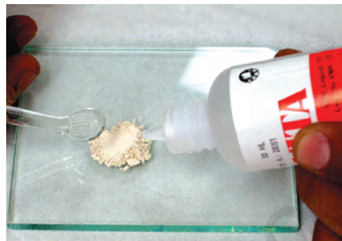
Figure 21.7: Opaquer powder is mixed and applied to hide the metal. It is mixed with the liquid to produce a sandy mix. A glass spatula is used for mixing as metal might abrade and contaminate the porcelain.
