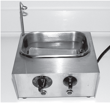
Figure 11.3: A thermostatically controlled water bath. This water bath maintains a steady softening temperature and is ideal for softening impression compound.
