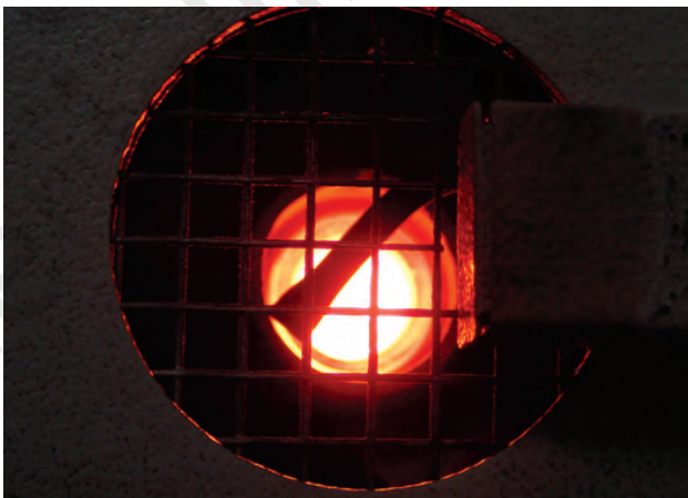
Figure 18.7: White hot molten alloy in crucible surrounded by the induction coil.
