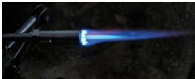
Figure 23.4: A neutral or reducing flame is used.
