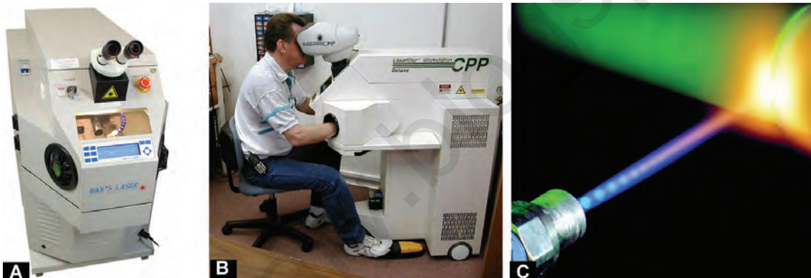
Figures 23.6 A to C: (A) A Laser welding unit. (B) A laser unit in operation. (C) Close-up of laser welding process.
