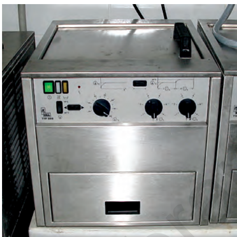
Figure 25.17: An automated curing bath (Kavo). The time and temperature of the curing cycle can be preset and regulated for optimum cure.
