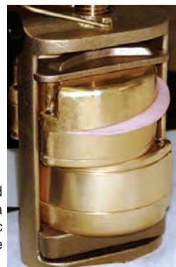
Figure 25.16: Assembled flasks after final closure in a holding clamp. (Excess acrylic called flash is evident in the picture).
