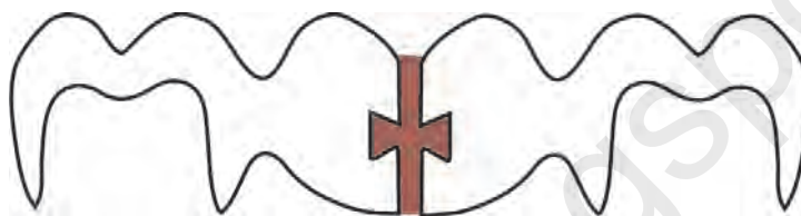
Figure 23.7: A mechanical interlocking design between two parts joined by cast-metal.
