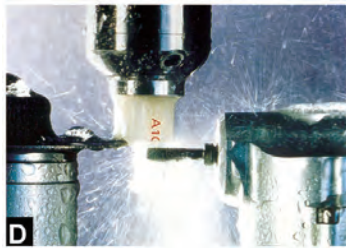
D The design is transferred to the milling station and A restoration is milled
