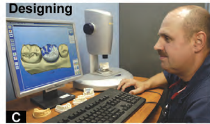
C A computer aids in designing the final restoration or coping
