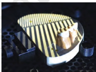
Figure 21.31: Light beam scanner (Kavo Everest).
